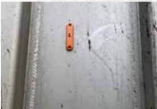
Example of an RFID Tag fitted to a vehicle
