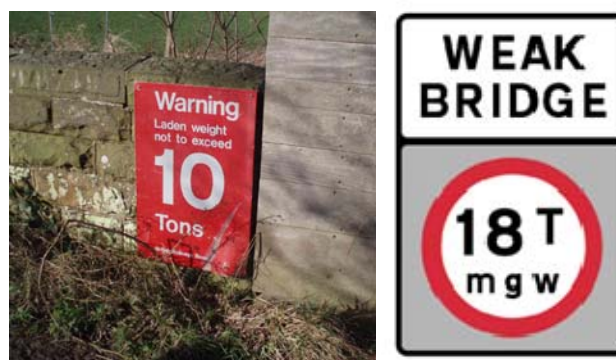
Figure 7 – Typical Maximum Weight restriction Signs
