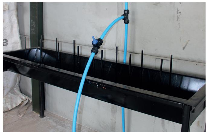
Chemical washing sink with drainage into biobed
