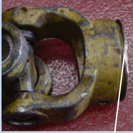
PTO yoke – damaged bearing groove.
